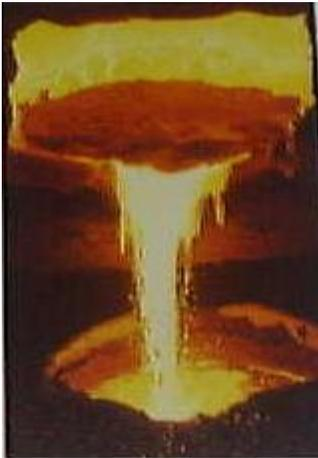
Molten gold being poured from a crucible into a vessel
