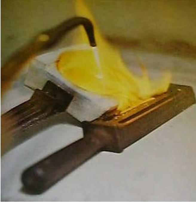
a crucible into mould
